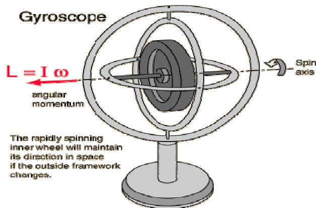
**Fig. 2:** A gyroscope: its structure and function
